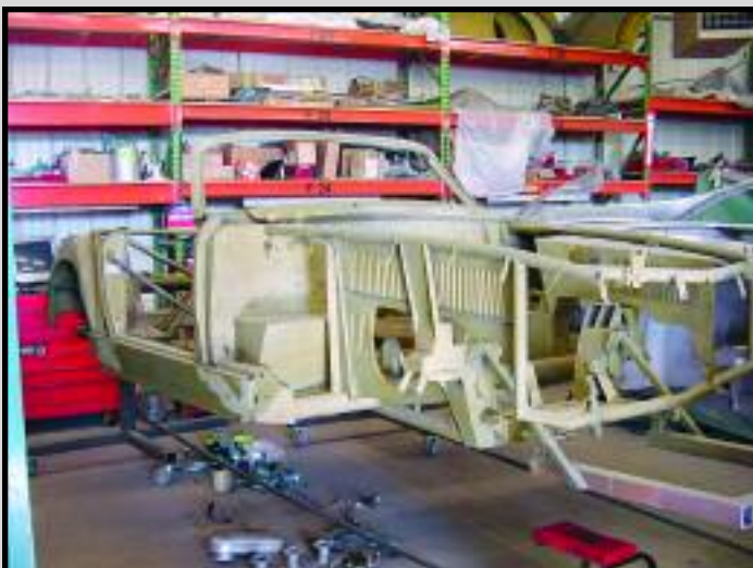
Chassis after assessment and light coat of etch prime to keep from flash rusting.
