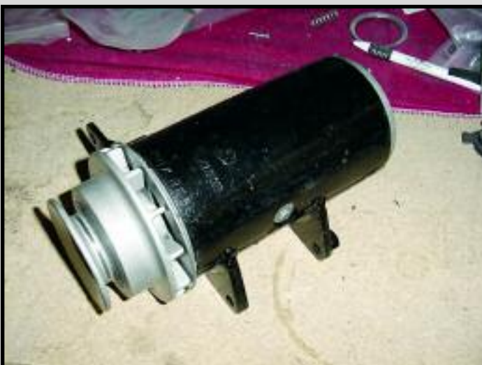
Original Marelli Dynamo after full rebuild, including field coil and armature rewind.
