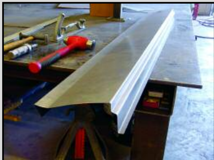
Newly fabricated rocker panel assembly.
