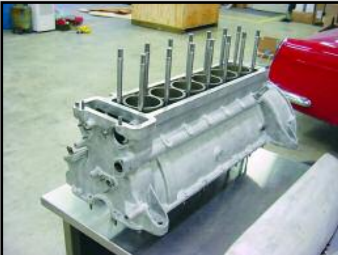
Showing prepared engine block.
