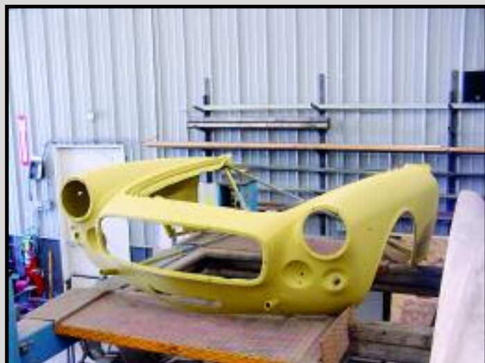
Nose assembly after primer coat ready for re-installation.
