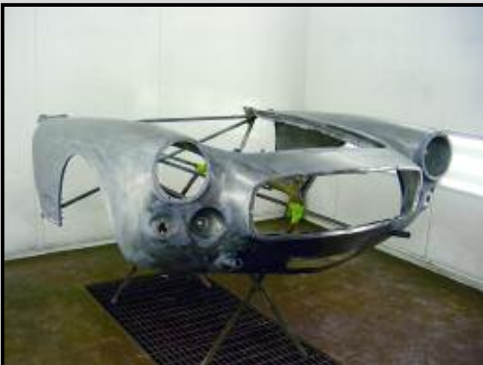
Front nose section with all metal work and straightening completed.
