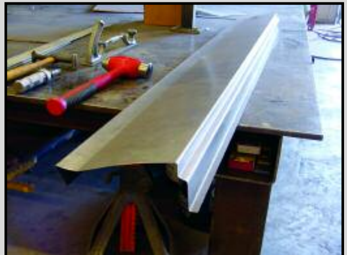
Newly fabricated rocker panel assembly.
