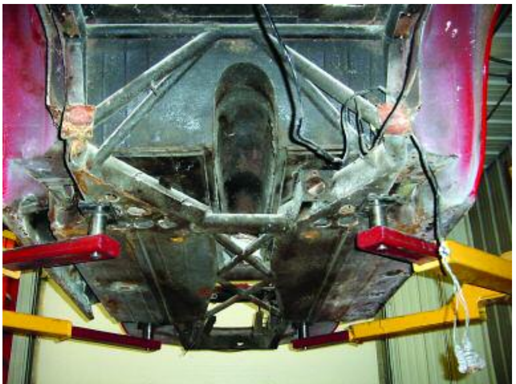
Primary chassis and forward structure found in remarkably solid condition.
