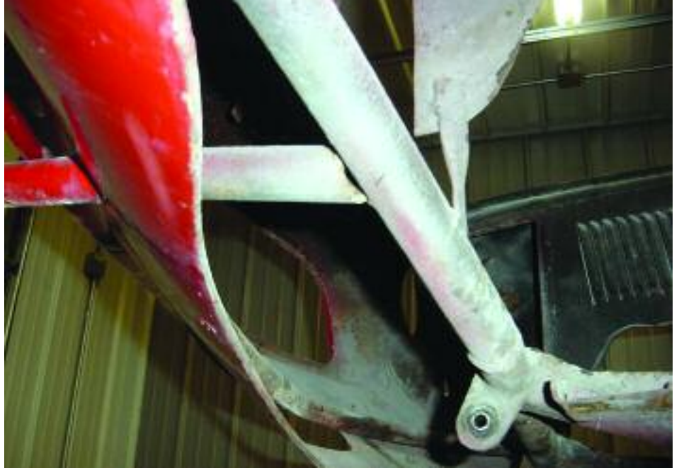
Front bumper frame extension only partially welded from the factory.
