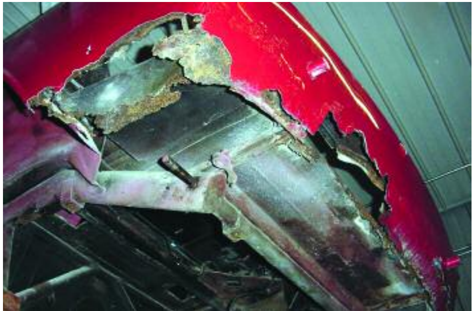
Evidence of serious rot and corrosion damage in rear structure/body.
