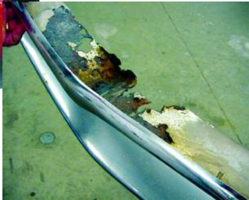
Front grill shell found to be the only trim piece in need of significant repair.
