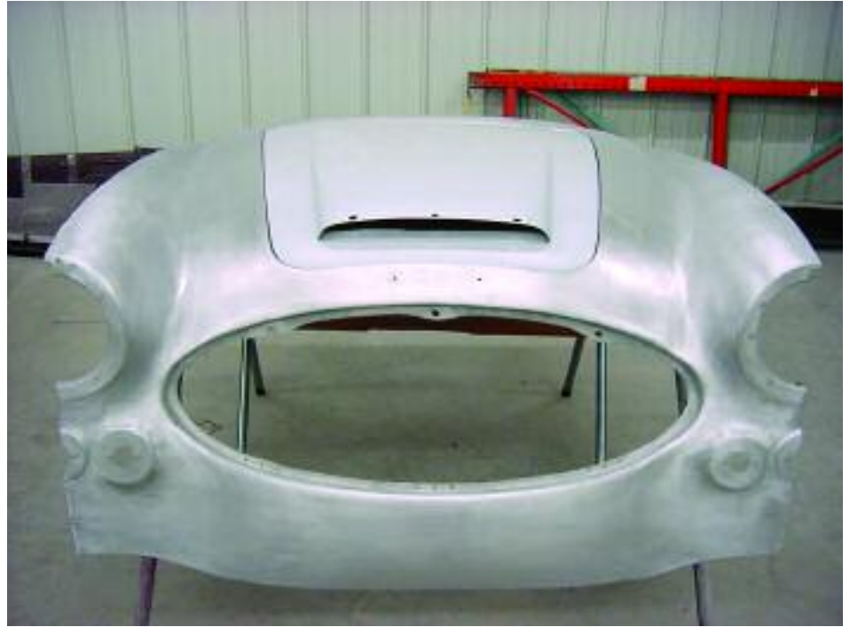
Healey 3000 front hood being fitted to front clip. This ensures proper fit in the final assembly stage.
