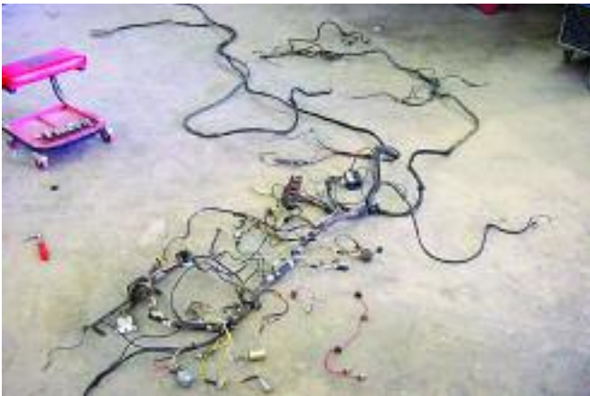
What a mess! Original wiring harness from Maserati 3500.
