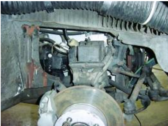
Maserati 3500 right front suspension before disassembly.
