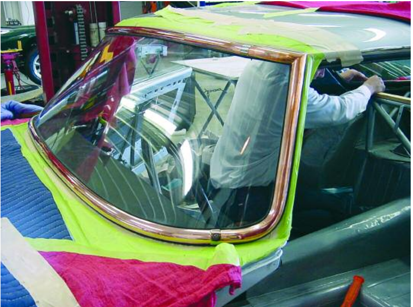
Below: Maserati 3500 windshield prefit of trim, in copper prior to chroming. This is done to ensure proper fit prior to sending the trim for chroming.
