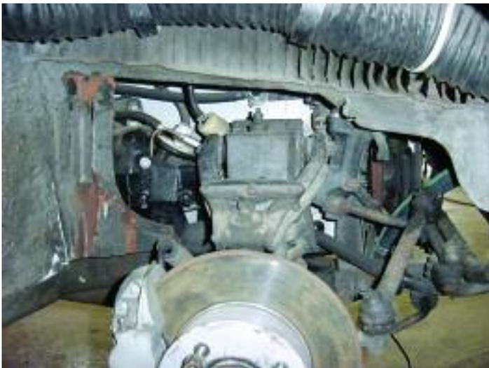
*Maserati 3500 right front suspension before disassembly.*
