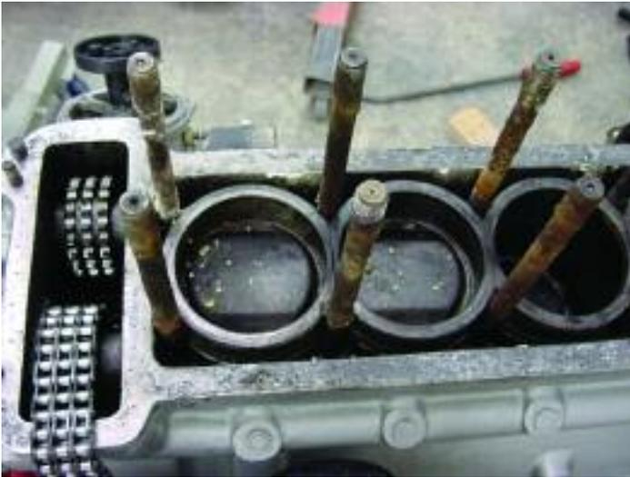
*Maserati 3500 Engine in disassembly process.*
