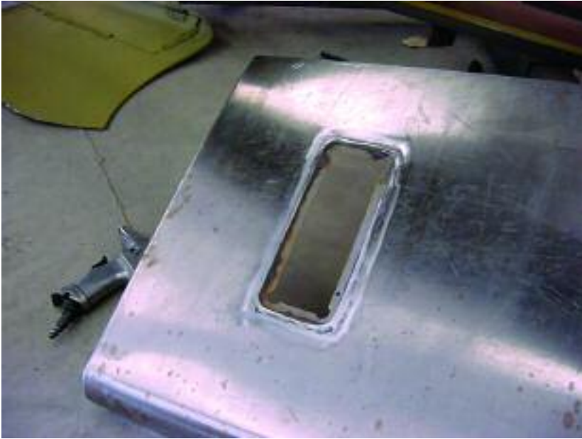
Jaguar XK 140 fender being remade.
