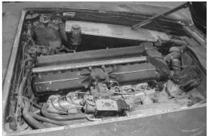
Note the original, intact, Lucas fuel injection system still on this car.
